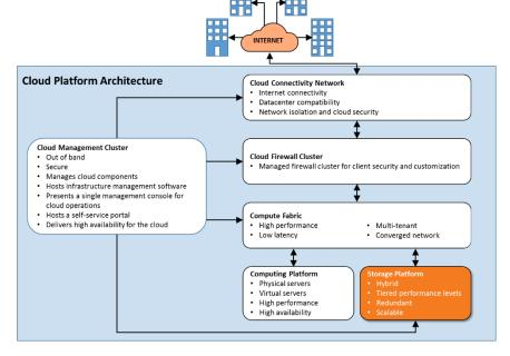
with servers over redundant 10Gb connections. Each storage array is fully redundant with automated availability features to maintain access to storage resources. All storage volumes are protected by RAID technologies to assure data high availability. All mirroring and retention of data is performed and retained on site in each cloud datacenter.
