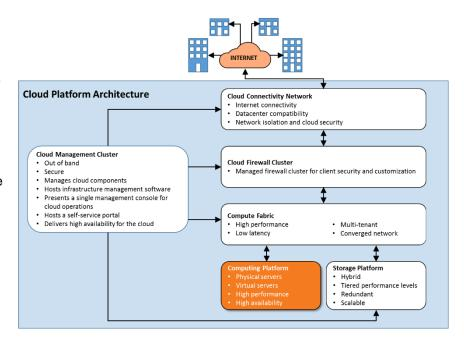
All VM host and physical servers connect to enterprise class shared, high-performance storage area network (SAN) storage via the high speed, low latency compute fabric.
